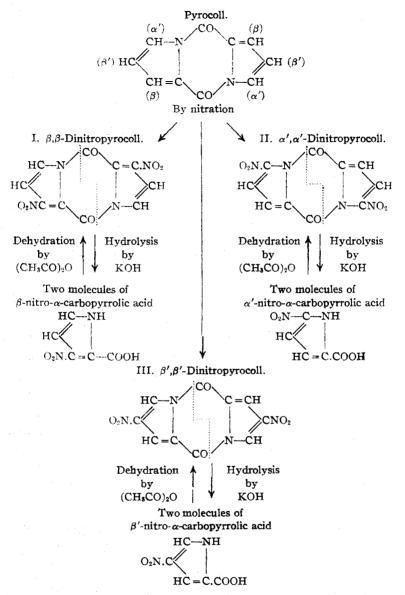
Further, in order to check this interpretation, we have reconverted the  $\beta$ -nitro- $\alpha$ -carbopyrrolic acid into this  $\beta$ ,  $\beta$ -dinitropyrocoll of Ciamician and Danesi. The method was suggested by the known action of acetic anhydride upon  $\alpha$ -carbopyrrolic acid, from which Ciamician and Silber were able to prepare pure pyrocoll. In the case of  $\beta$ -nitro- $\alpha$ -carbopyrrolic
